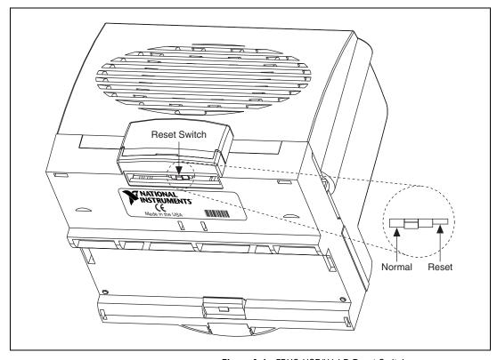
Figure A-1. FBUS-HSE/H1 LD Reset Switch
